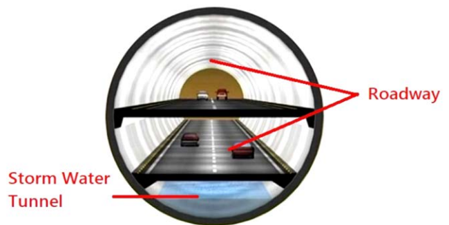
Cross-Sectional View of the SMART Tunnel
